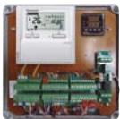
AHU kit. PCB, power transformer, terminal block
